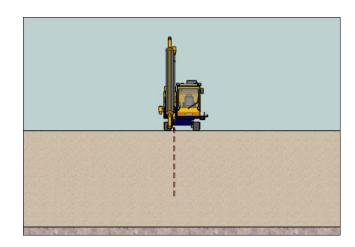
Operator moves machine to drill mark and sets up x- and y-angle to desired values (e.g. 20° / 0°).
